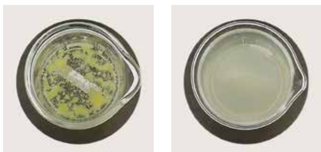
Fig. 3: Use of PHOSAL® H 50 to emulsify dietetic oils. Left: Pure fish oil in water. Right: mixture of 70 % fish oil and 30 % PHOSAL® H 50 mixed with water forming emulsion droplets.
